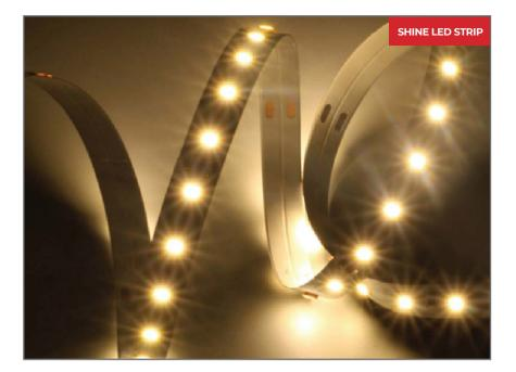
SHINE LED STRIP Flexible LED strip lighting designed to create a smooth wash of ambient and vertical illumination between wall and ceiling planes. Powered by high-quality LEDs with a binning tolerance of  $\leq$  3 SDCM and CRI  $\geq$  90, ensuring vibrant and accurate color rendering. The strip maintains at least 70% of its luminous flux after 50,000 operating hours, guaranteeing long-term performance and reliability.
